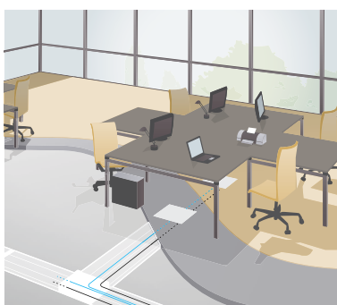
Screed floor system
